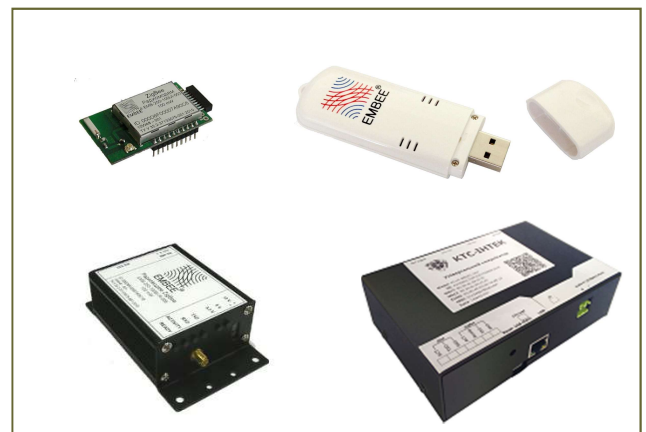
Fig.2 The components of mesh network is Embee modems with embedded software and AT command and Data aggregator unit with Ethernet/3G communication to WAN.
